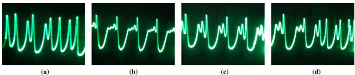
Fig. 22 Experimentally captured coexisting firing patterns with R_B = 24.99 \text{ k}\Omega . a Chaotic spiking firing. b Periodic bursting firing. c Chaotic bursting firing. d Transient chaotic bursting firing. (Color figure online)
