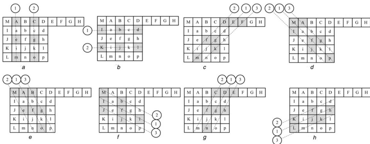
**Fig. 4** Orientation gradients of the directional modes for I4MB, (a) and (b) responding to mode 0, 1, 3, ..., 8
