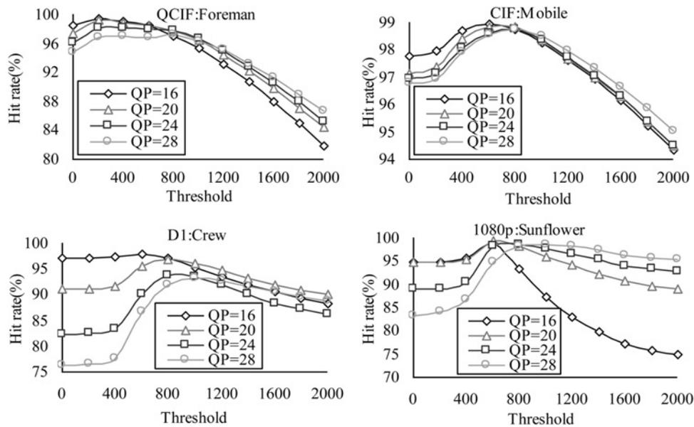
**Fig. 3** Hit-rates of different DTV thresholds for various resolution sequences under four QPs
